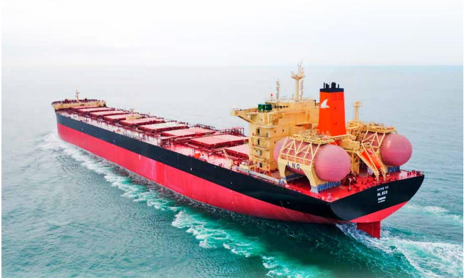
In 2020, Panama flagged the world's first LNG-powered bulk carriers, HL Green and HL ECO operated by H-Line Shipping. The vessels have a cargo capacity of 180,000 DWT and are 292 m length overall, 45 m breadth moulded and 18.0 m draught.
